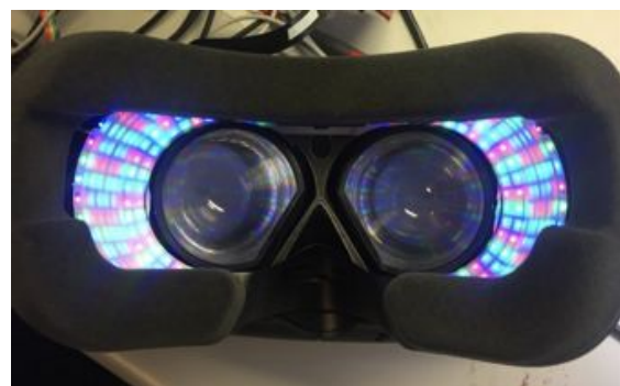
Figure 3: HTC Vive with a Sparse Peripheral Display extending the FOV to 180°.
